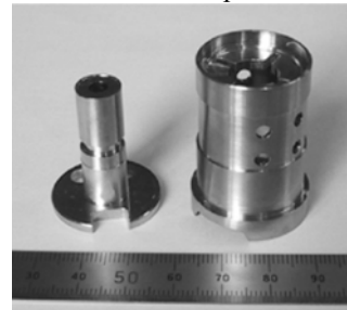
Example of application (injector core parts for use in LPG vehicle)
